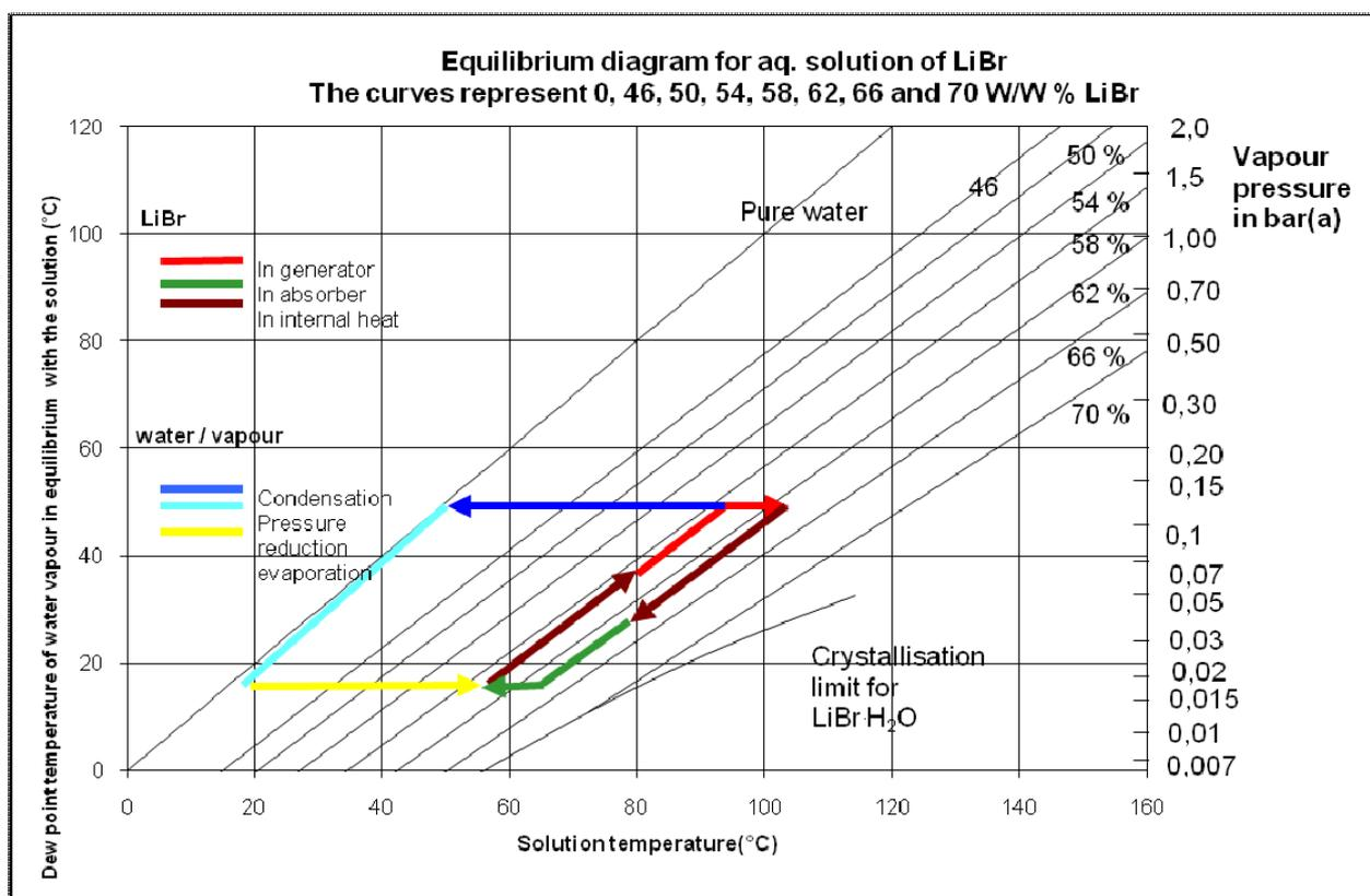
As an example, pure water at 20 °C has a vapour pressure of 0,0234 bar(a). At the diagram, it can be seen that the vapour pressure is the same for a 58 % aqueous solution of Lithium bromide at 57 °C or a 62 % solution at 66 °C. It can be mentioned that the vapor consists of pure water vapor. The salt (Lithium Bromide) does not evaporate at all.
