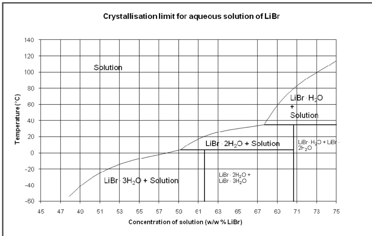
However, crystallisation rarely occurs and normally it does not give any damages of the machines.
